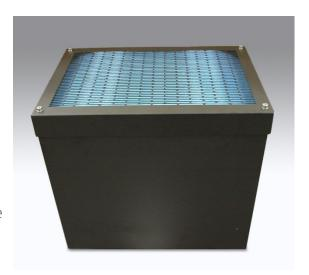
GEW supply an ozone filter capable of destroying ozone. Each filter cell is manufactured from transparent Makrilon to withstand temperatures of up to 115°C. The life span of the media is fairly long due to the catalytic process that occurs and media replacement should be determined by colour change from purple to light brown.
